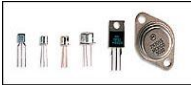
Typical transistor packages
