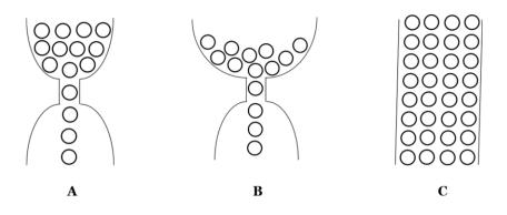
Figure 6.4 - A) visualisation of a bottleneck situation, B) process improvement, but the bottleneck has not been addressed, and C) situation without a bottleneck
