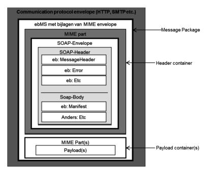
Figure 7.12 – Structure of an ebMS message
