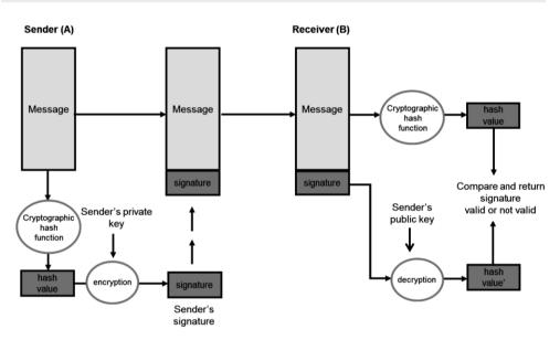
Figure 8.5 – Simplified depiction of using a cryptographic hash function to create a digital signature for authentication purposes (based on Stallings, 2011)
