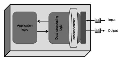
Figure 7.10 – Elements of a web service (based on Erl, 2008)
