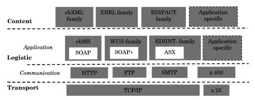
Figure 7.8 - Typical standards for the design and implementation of interfaces
