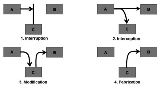
Figure 8.3 – Typology of man-in-the-middle attacks (by malicious party C) that may occur during electronic data interchange between A and B
