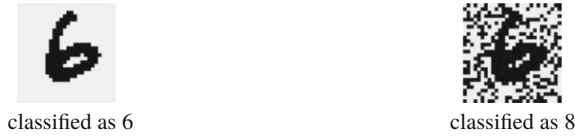
Fig. 10 Adversarial changes identified by DF after 60.89 h by fuzzing up to 50% pixel changes for a fixed image. The learned model classifies the left (original) image as a 6, while it classifies the right image as an 8. The images differ in 314 pixels
