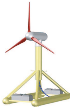
Figure 3. Example of TEC used for manual installation and maintenance maneuvers. Additional details about this TEC design can be found in [38].
