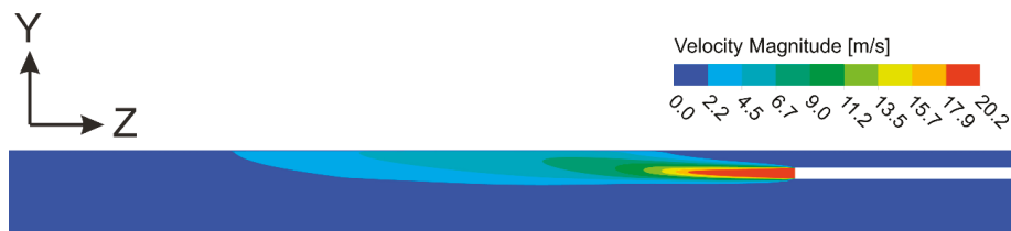
Figure 7. Velocity contours of the air jet exiting the ventilation duct along the tunnel axis. The data correspond to scenario 4 and 20 m/s air velocity at the velocity inlet.
