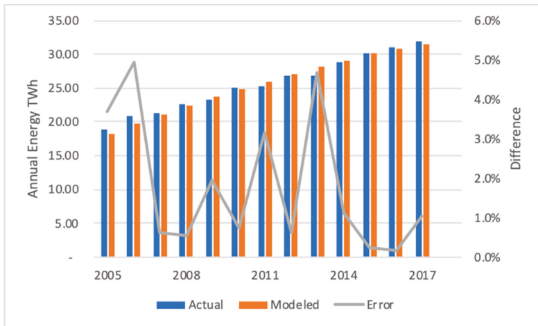
Figure 7. Comparison of the actual and modeled annual residential sector energy use from 2005 to 2017.
