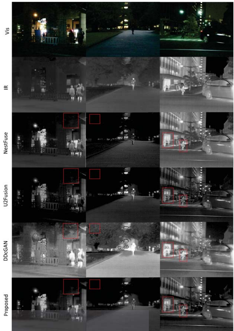
Figure 2. Qualitative comparison of the proposed method with other state-of-the-art methods on image pairs taken from the private dataset. The first row contains visible images. Second row contains infrared images. The last row contains the fused results of our proposed method.
