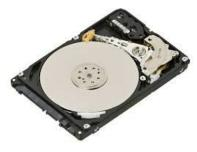
Drives with a capacity less than 1 Terabyte usually have just one platter. Notice the single platter in the image. The read/write arm must be positioned over the appropriate track before accessing or writing data.
